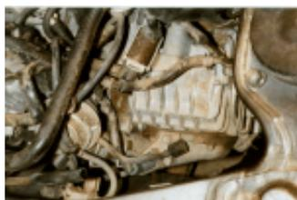
The radiator overflow tank has been removed. The Air Vent Control valve is the brown one on top of the supercharger with three hoses attached to it. The ABV diaphragm control valve is the blue valve near the bottom with a hose running to the AVB. The brown valve in the very bottom vents the fuel pressure regulator's compensation port to the atmosphere.
